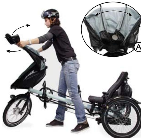
4. Hold the outer edges of the fairing frame, and spread the fairing apart as shown (Fig. A).
